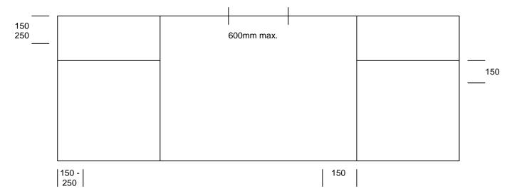
Secure the frame by whichever method ensuring not to overtighten the fixing, packers should be fitted adjacent to the fixings to hep prevent distortion of the outerframe.
