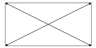
If the aperture diagonals are more than 10mm out of each other, use of a straight edge to determine the usable area of the aperture. Then measure the width and height of the remaining aperture.
