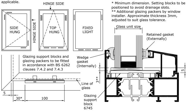
In Hi+ applications only 6727 glazing unit perimeter foam to abut 6745 glazing support.
