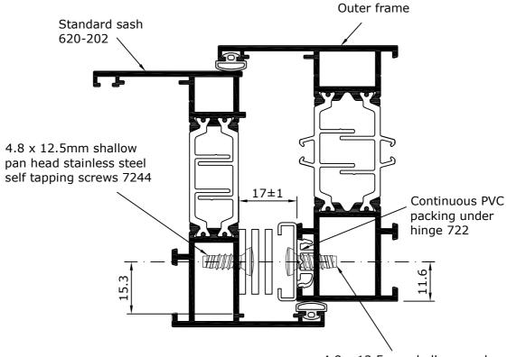
4.8 x 12.5mm shallow pan head stainless steel self tapping screw 7244. (Use vee in section to locate drill for screw pilot holes).
