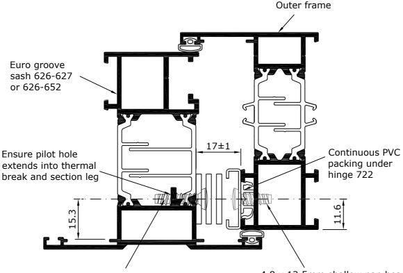
4.8 x 18mm shallow pan head stainless steel self tapping screws 7245 or No 8 x 19mm countersunk stainless steel self tapping screws 7231 when 6708 hinge is being used.
