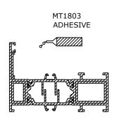
MT1803 ADHESIVE SHOULD BE APPLIED TO THE PERIMETER OF THE CLEAT CHAMBER OF THE FRAME SECTION AND THE CORNER BRACE GROOVE.
