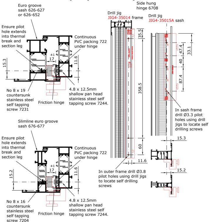
Euro Groove Sashes 626-627 and 626-652 Fixing Positions for 6709 Hinges
