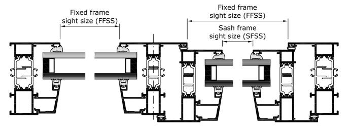
The fixed frame sight size can be calculated from the "Ready Reckoner", the section drawings or dimensioned general arrangement drawings provided.
