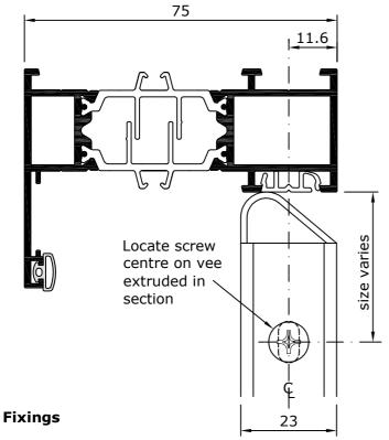
For hinges 6705, 6706, 6707 and 6709 use austenitic stainless steel shallow pan head self tapping screws 7244 and 7245 to fix vent arm and track as shown on the following pages. For hinge 6708 use countersunk screws to vent arm and screw 7244 to track.
