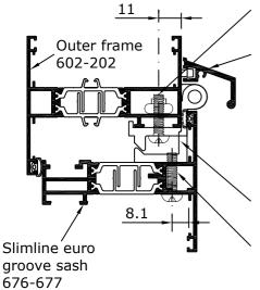
3 No. M5 x 20mm pan head stainless steel fixing screws 7208 into M5 countersunk aluminium rivnuts 7209
