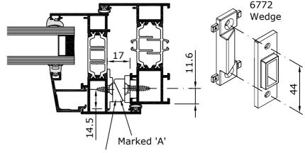
Alignment wedges 6772 to be provided at jambs of top hung sash and head and cill of side hung sash (near to leading edge). To be fixed with 2 No 8 x 19mm countersunk head screws 7231 to outer frame and 2 No 8 x 12mm countersunk head screws 7230 to sash.
