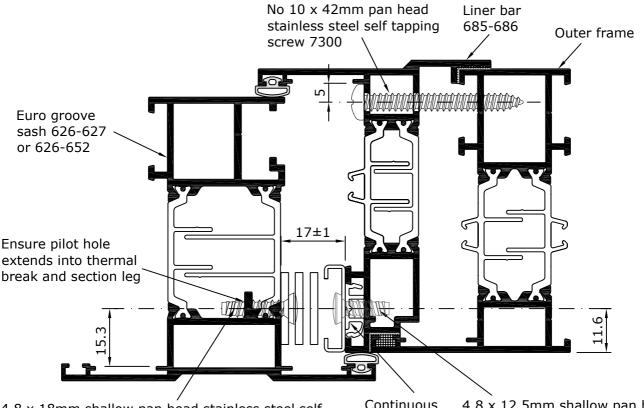
4.8 x 18mm shallow pan head stainless steel self tapping screws 7245 or No 8 x 19mm countersunk stainless steel self tapping screws 7231 when 6708 hinge is being used.
