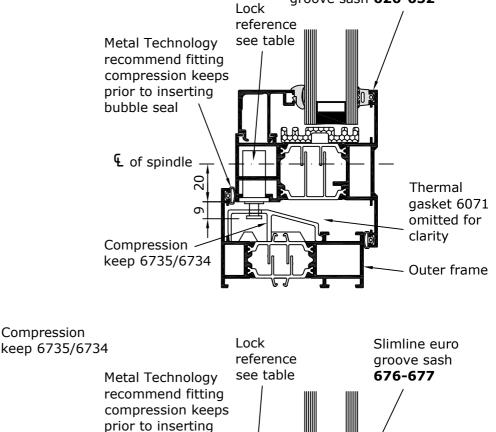
In Hi+ applications 6071 gasket to be bonded to outer frame using HR50328A sealant
