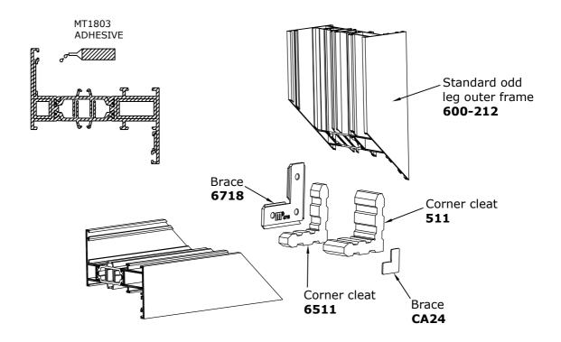
MT1803 ADHESIVE SHOULD BE APPLIED TO THE PERIMETER OF THE CLEAT CHAMBER OF THE FRAME SECTION AND THE CORNER BRACE GROOVES.
