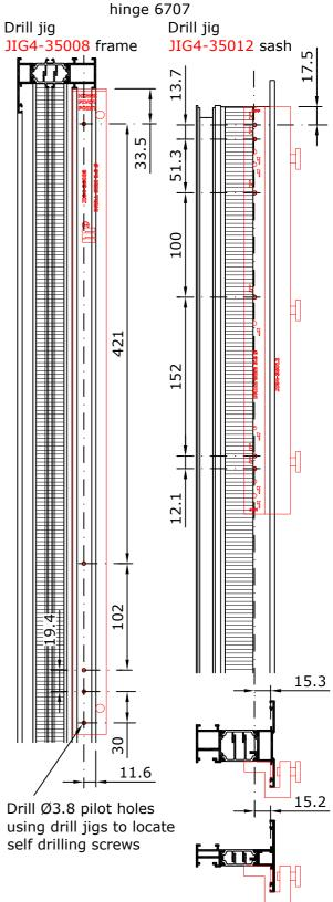
Euro Groove Sashes 626-627, 626-652 and 676-677 Fixing Positions for 6708 Hinge
