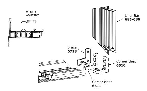
MT1803 ADHESIVE SHOULD BE APPLIED TO THE PERIMETER OF THE CLEAT CHAMBER OF THE FRAME SECTION AND THE CORNER BRACE GROOVE.
