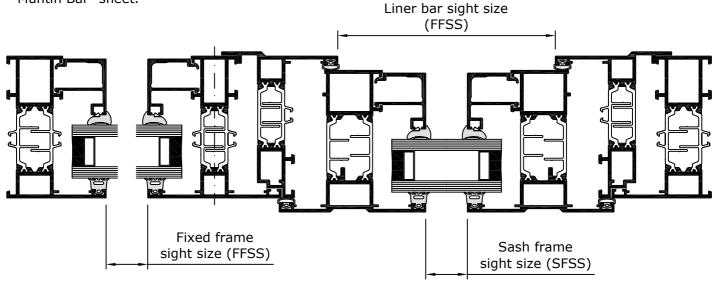
When calculating the sash size in liner bar applications the fabrication datum is measured from the "Liner bar sight size" (LBSS) as indicated.
