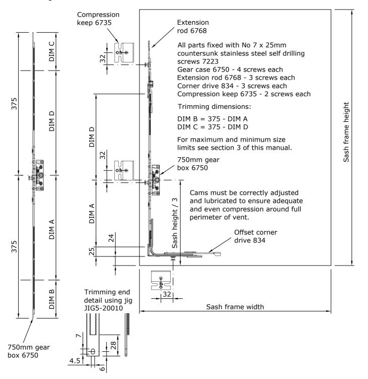
Side Hung Window Euro Groove Sashes 626-627 and 626-652 Sash Heights 1016mm to 1303mm with Handle at 1/3
