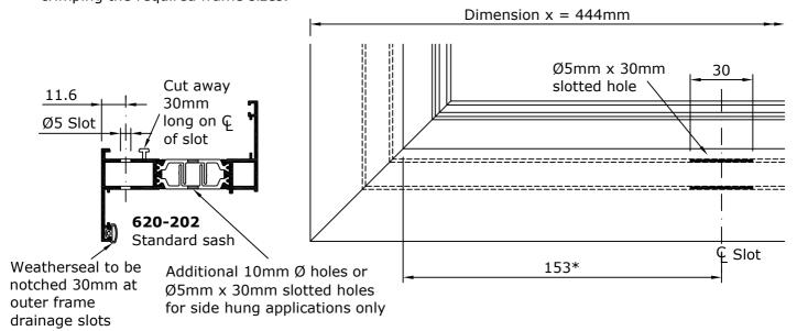
Additional 10mm Ø holes or Ø5mm x 30mm slotted holes for side hung applications only
