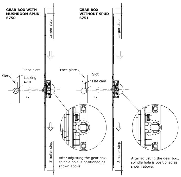
When using rods/extensions 844, 845, 6767, 6768 ensure locking/flat cam is centred in 43mm slot of face plate prior to cropping.
