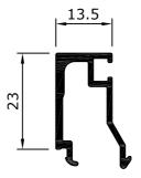
653 44mm/47mm SQUARE GLAZING BEAD (not suitable for use with slimline sash 676-677)
