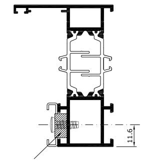
2 No hinge supports 504 per pair of jamb hinges, each fixed with 2 No 4.8 x 12.5mm shallow pan head stainless steel self tapping screws 7244
