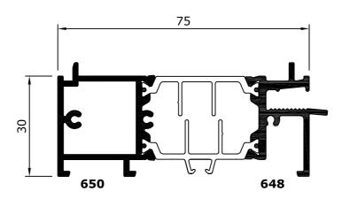
650-648 MEDIUM FLUSH CILL LINER (FOR PRESSED METAL CILL) (Not suitable for use with coupling mullions)
