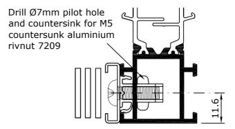
Secure restrictor plate within the outer frame track of the friction hinge at the "Maximum opening angle" in accordance with "Friction Hinges - Hinge Restrictor Plate Fixing" sheet.
