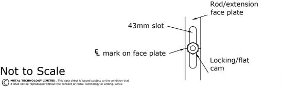
Side Hung Window Euro Groove Sashes 626-627 and 626-652 Sash Heights 500mm to 677mm with Handle at Mid-point
