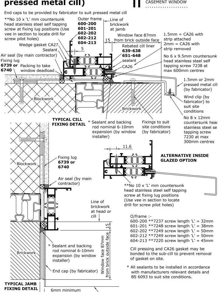
Scale 1:2 METAL TECHNOLOGY LIMITED. This data sheet is issued subject to the condition that it shall not be reproduced without the consent of Metal Technology in writing. 02/10 1.5mm or 2mm pressed metal cill (by fabricator)
