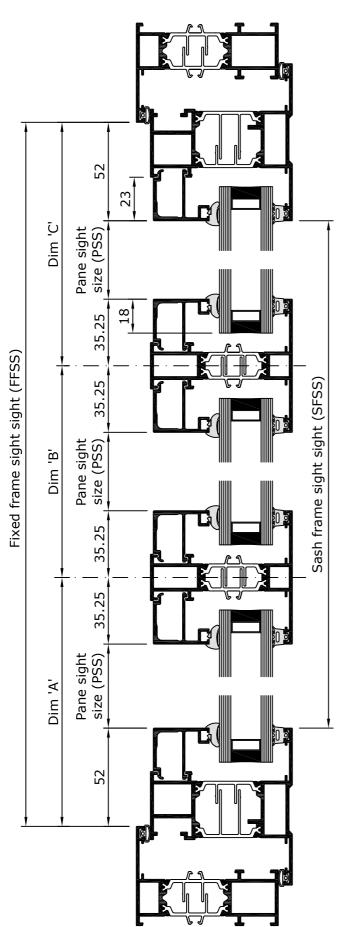
All cutting sizes for beads and glass into sashes with muntin bars are to be calculated using pane sight sizes (PSS).
