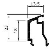
654 44mm/47mm RAKED GLAZING BEAD (not suitable for use with slimline sash 676-677)
