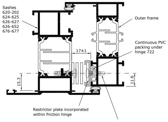
For hinges 6705, 6706, 6707, 6709 restrictor plates must be secured, through pre-drilled holes in hinge track, using No 7 x 16mm countersunk self drill screws 7256. Restrictor plate position to be determined according to applicable sash weight.
