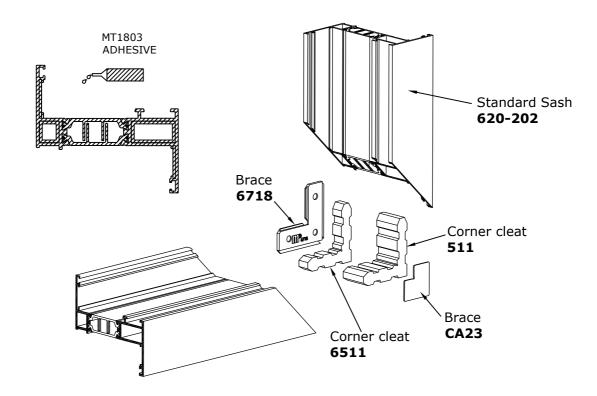
MT1803 ADHESIVE SHOULD BE APPLIED TO THE PERIMETER OF THE CLEAT CHAMBER OF THE FRAME SECTION AND THE CORNER BRACE GROOVE.
