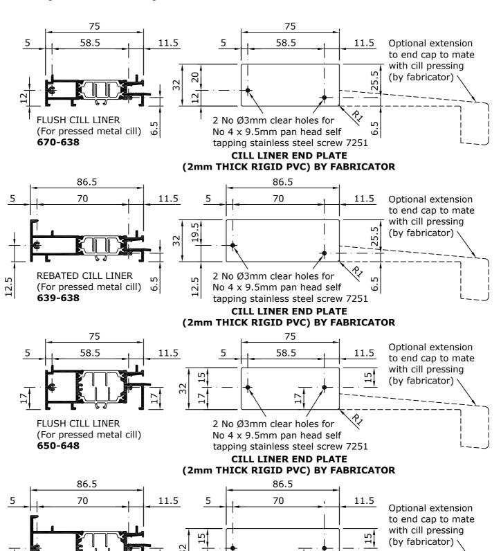
**CILL LINER END PLATE** (2mm THICK RIGID PVC) BY FABRICATOR
