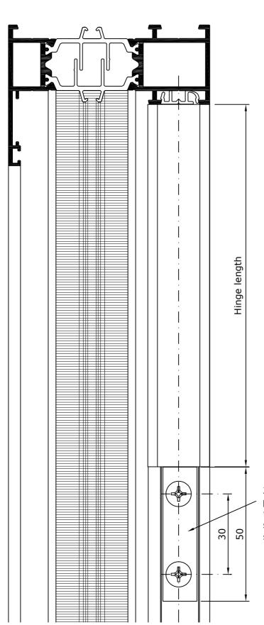
Hinge support blocks must be used for all factory glazed windows to reduce the risk of vents dropping during transportation and installation. They are not a substitute for careful handling.
