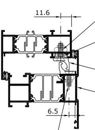
2 No M5 countersunk aluminium rivnuts 7209 with M5 x 16mm stainless steel countersunk machine screws 7227 located at position shown.
