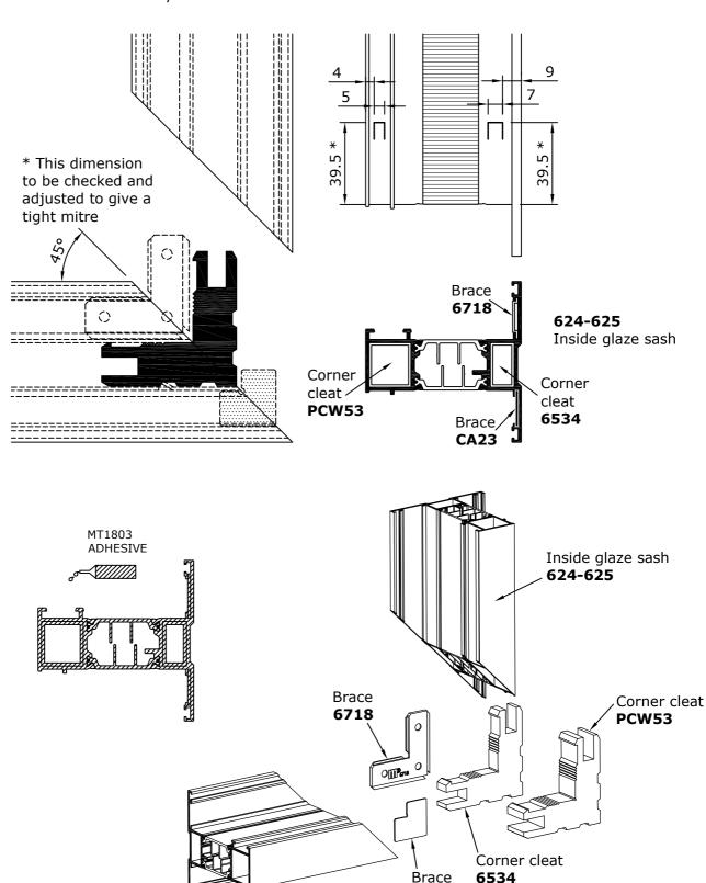
MT1803 ADHESIVE SHOULD BE APPLIED TO THE PERIMETER OF THE CLEAT CHAMBER OF THE FRAME SECTION AND THE CORNER BRACE GROOVE.
