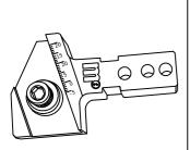
CR124303800/MOD ADJUSTABLE TOOL HOLDER FOR EP124 CRIMPER
