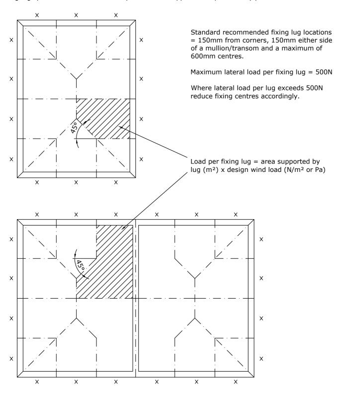
NOTE: Fabricator to ensure that the fixing to the structure and the structure itself is also capable of withstanding the imposed loads (i.e. wind load and dead load).
