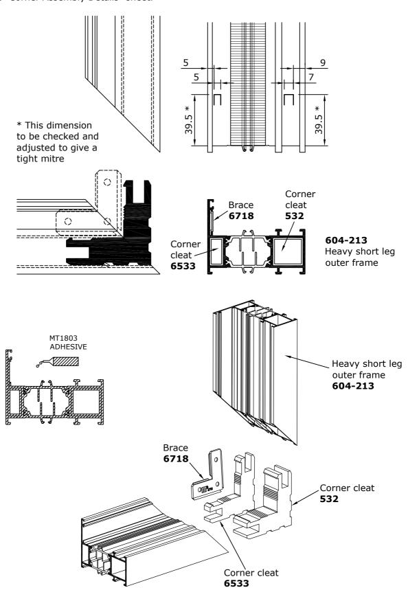
MT1803 ADHESIVE SHOULD BE APPLIED TO THE PERIMETER OF THE CLEAT CHAMBER OF THE FRAME SECTION AND THE CORNER BRACE GROOVE.
