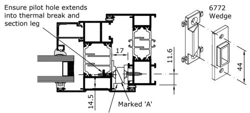
Alignment wedges 6772 to be provided at jambs of top hung sash and head and cill of side hung sash (near to leading edge). To be fixed with 2 No 8 x 19mm countersunk head screws 7231 to outer frame and 2 No 8 x 19mm countersunk head screws 7231 to sash.
