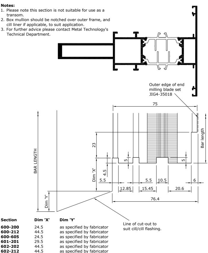
If 'Y' is specified as 0, bar will be square ended. Values of 'X' and 'Y' must be provided for both ends of the bar.
