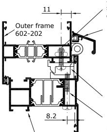
Recessed euro groove sash 626-627 or flat euro groove sash 626-652
