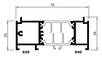
**650-040** FLUSH HEAD LINER (Not suitable for use with coupling mullions)
