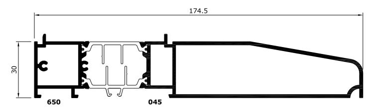
650-045 FLUSH SUB-CILL (Not suitable for use with coupling mullions)
