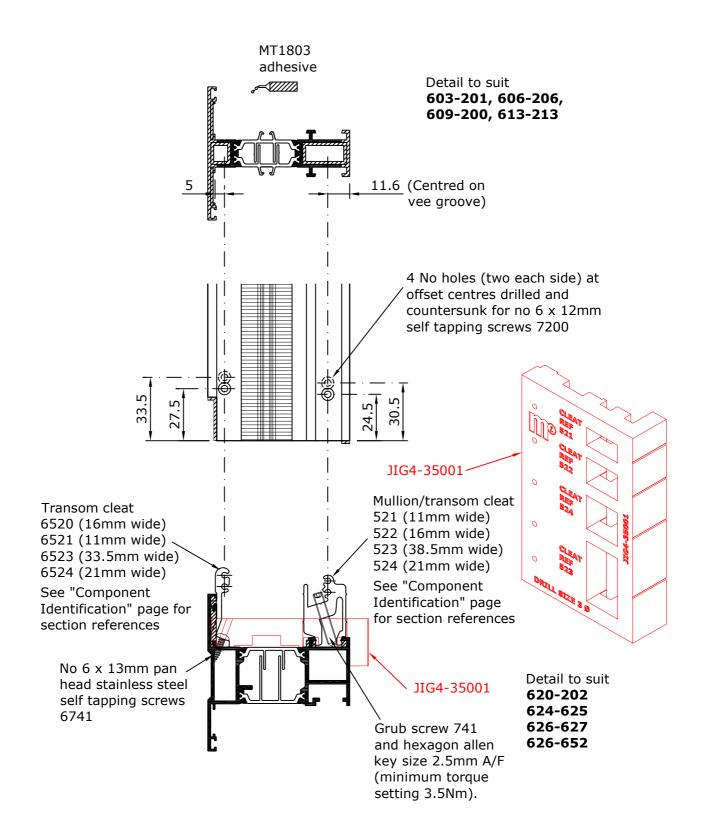
For isometric details of joint assembly and adhesive/sealant application see "Mullion/Transom Sealing Detail" sheet.
