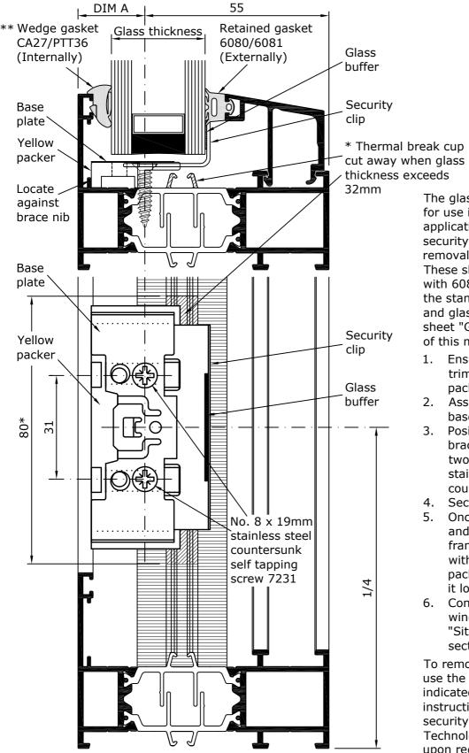
The glass security clip is designed for use in externally beaded applications to provide additional security against the unauthorised removal of the double glazed units. These should be used in conjunction with 6080/6081 captive gasket and the standard glazing support blocks and glass packers as detailed on sheet "Glazing Details" in section 8 of this manual.
